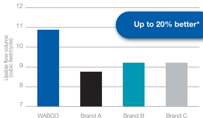
Usable flow volume is a measure of how much air flow the cartridge can process while still maintaining dry air
