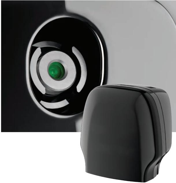
This Driver Tips Guide applies to vehicles equipped with the WABCO OnLaneALERT™ Lane Departure Warning System. OnLaneALERT is a camera-based warning system that helps drivers avoid unintentional lane drifting.
